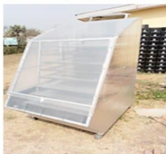
Figure 8b: Hybrid solar dryer positioned to receive optimum sun exposure
