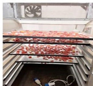
Figure 8c: Hybrid solar dryer loaded with tomato slices in single layers and adequate spacing
